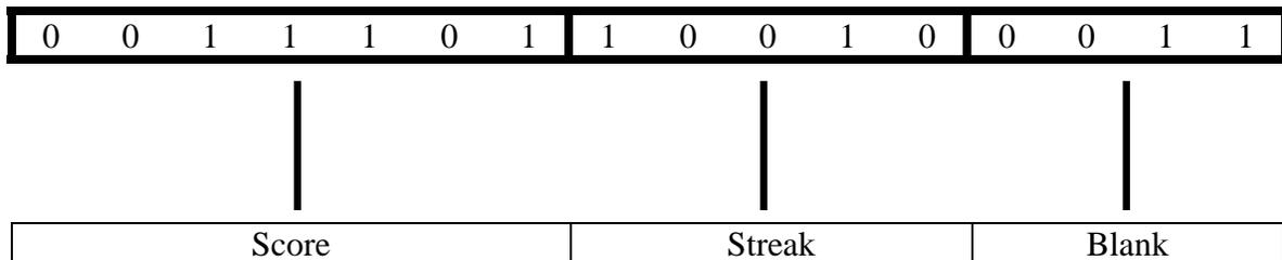
This packet is sent from software to hardware whenever a change occurs. The 7 bits of “Score” allows up to 127 points to be kept, where only 100 are used. “Streak” marks the longest streak of “Perfects” that the player has achieved so far.
