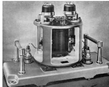
Magnetic drum memory. 1950s & 60s. Secondary storage.
