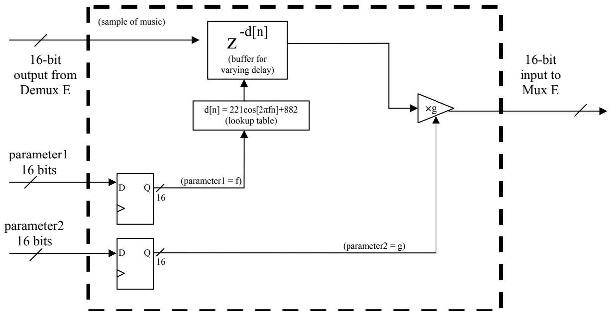
Fig. 4. Block Diagram of Vibrato Module
