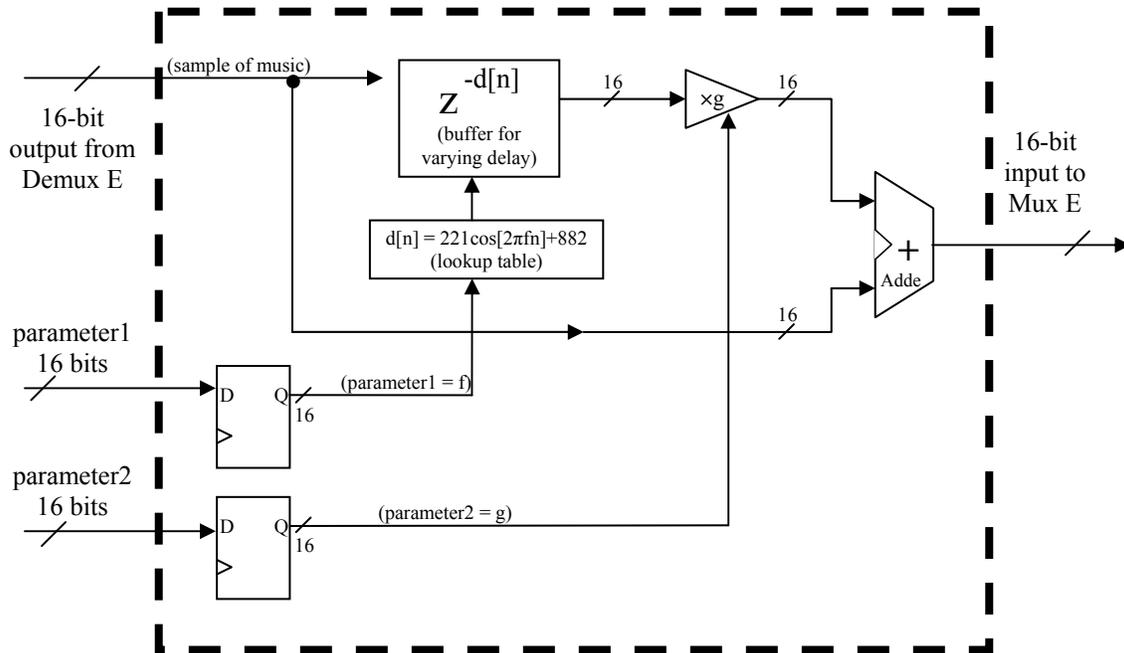
Fig. 5 Block Diagram of Chorus module
