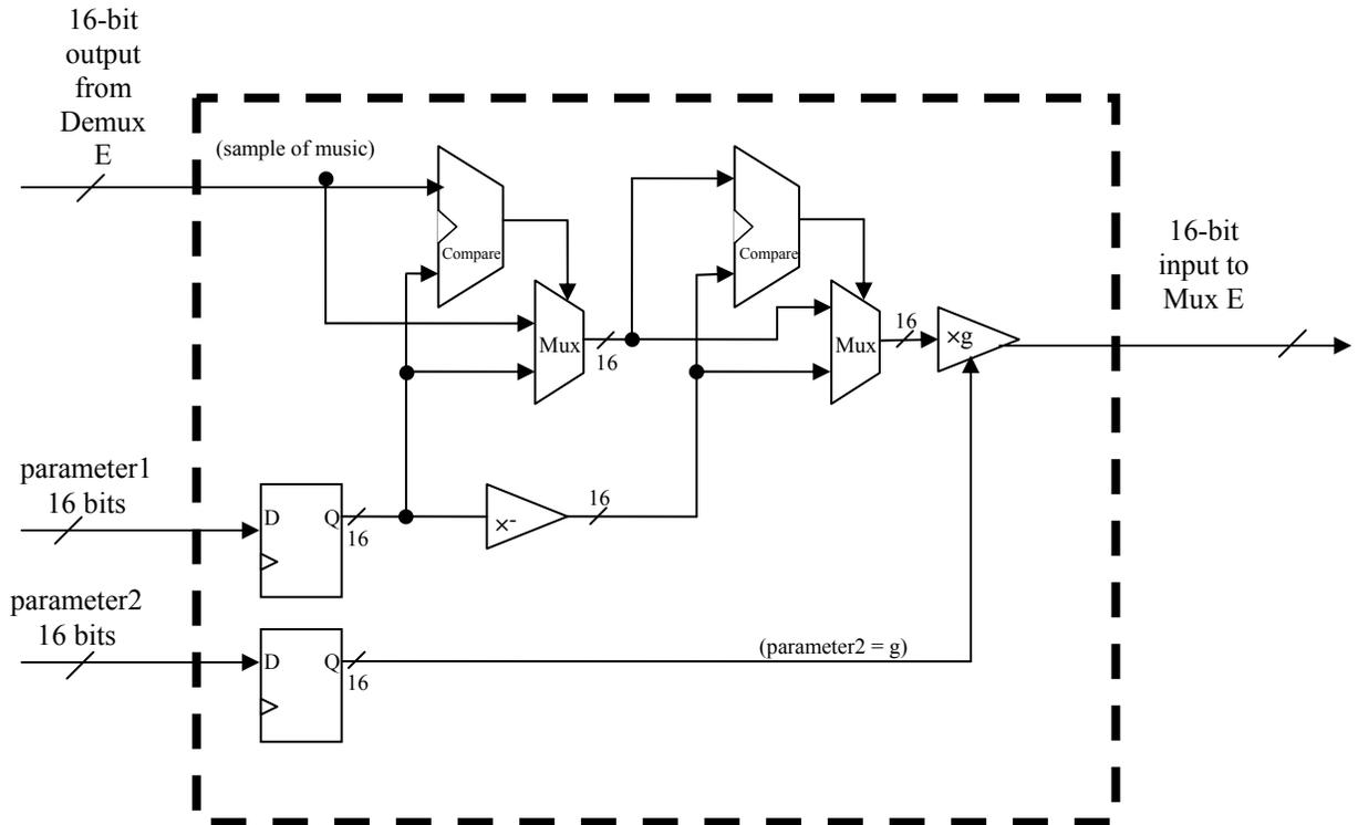
Fig. 3 Block Diagram of Distortion Module
