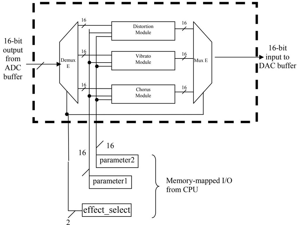
Fig. 2 Effects processor block diagram
