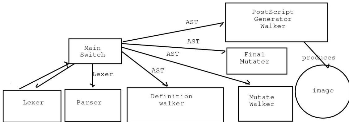
The Parser is also interesting in that it has to compare the values in the indentation tokens. Each indentation token has a value representing how deeply the subsequent statement is indented. That indentation needs to be compared with previous indentations to find where the subsequent statement belongs on the AST.
