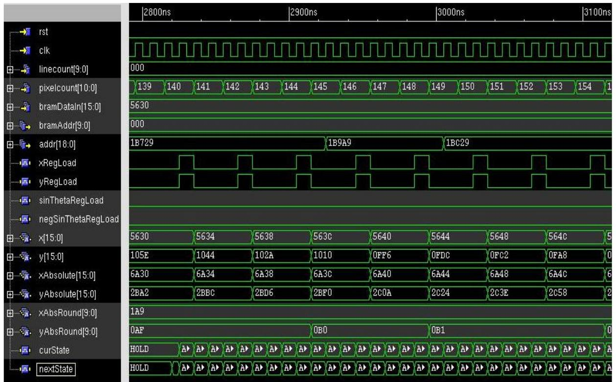
The next step was to test it in isolation in hardware. We hooked up an artificial BRAM and used the OPB to report the address output from the warper. The module (plus fake BRAM and OPB controls) compiled and ran in hardware, reporting correct address values for a number of specific points (pixel-count values) that we checked.
