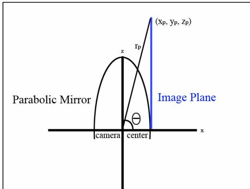
By parameterizing the arc traced out upon the (x,y) plane in terms of a rotation about a point on the plane, for each scanline, it becomes possible to iteratively calculate every point on a scanline, provided only with the first point on the scanline and the angle of increment.
