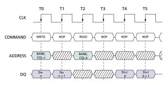
NOTE: The WRITE command may be to any bank, and the READ command may be to any bank. DQM is LOW. CAS latency = 2 for illustration.
