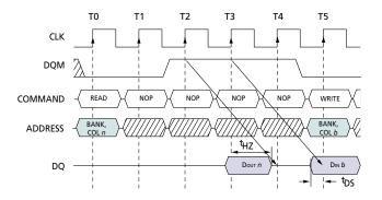
NOTE: A CAS latency of three is used for illustration. The READ command may be to any bank, and the WRITE command may be to any bank.
