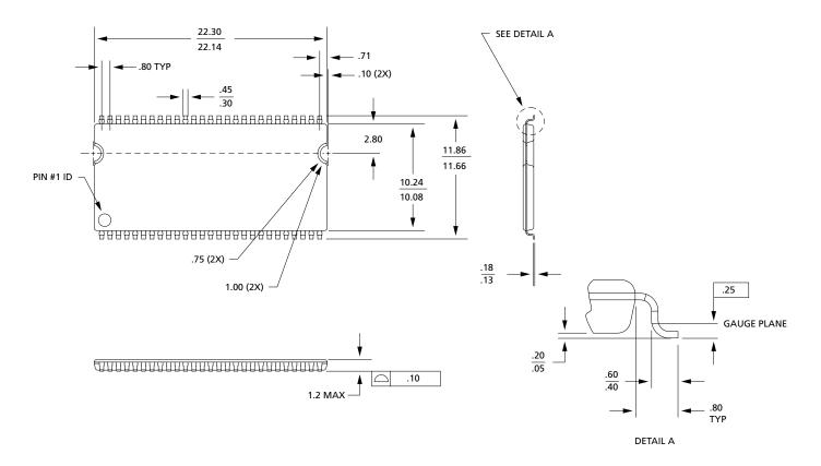
**NOTE:** 1. All dimensions in millimeters  $\frac{MAX}{MIN}$  or typical where noted.
