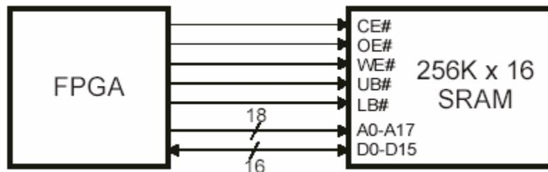
The SRAM was already configured for us. “Mylinkscript” defines which parts of software go in the SRAM. By following that, we were able to place out buffers in the SRAM.
