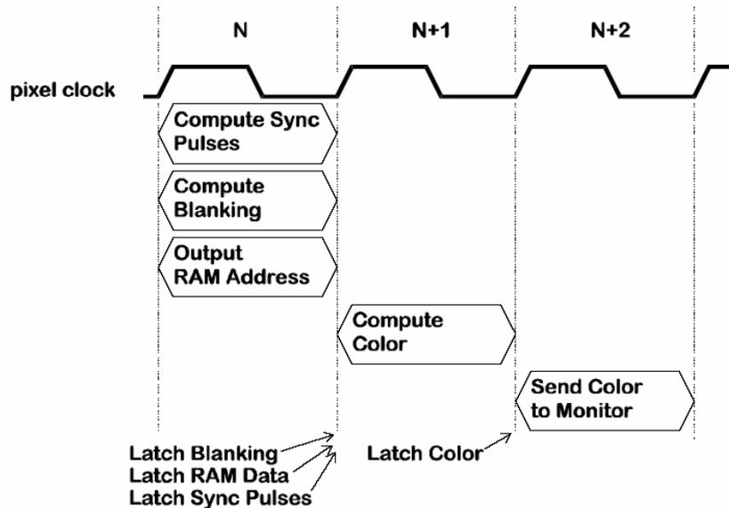
Figure 3: Pipelining of VGA signal generation tasks.
