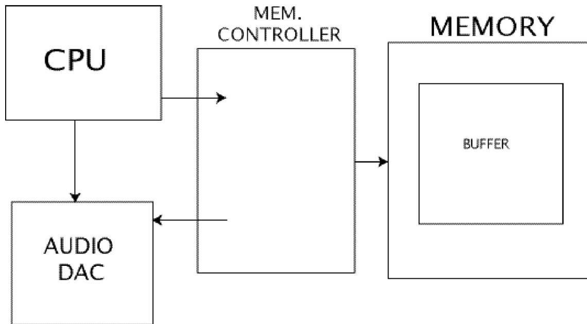
Figure 7: Memory Controller and Neighboring Components
