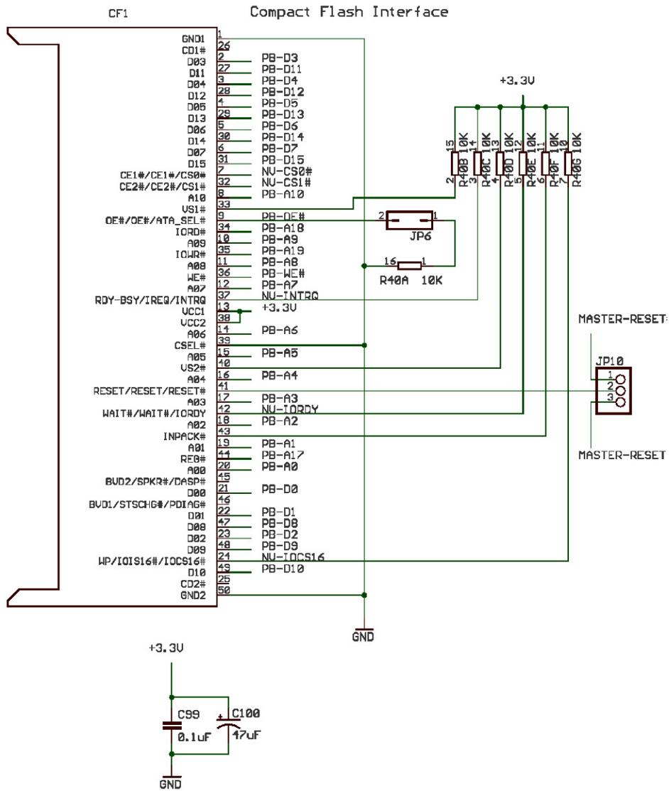
Figure 6: Mapping of the FPGA Pins to the CompactFlash Connector
