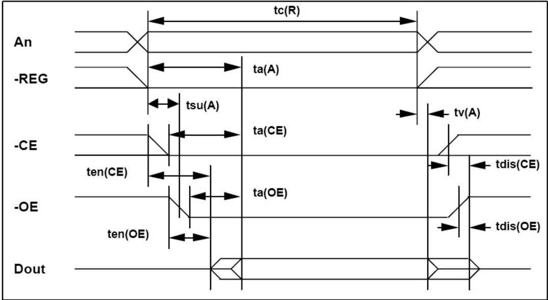
Figure 3: Timing Diagram of Attribute Memory Read
