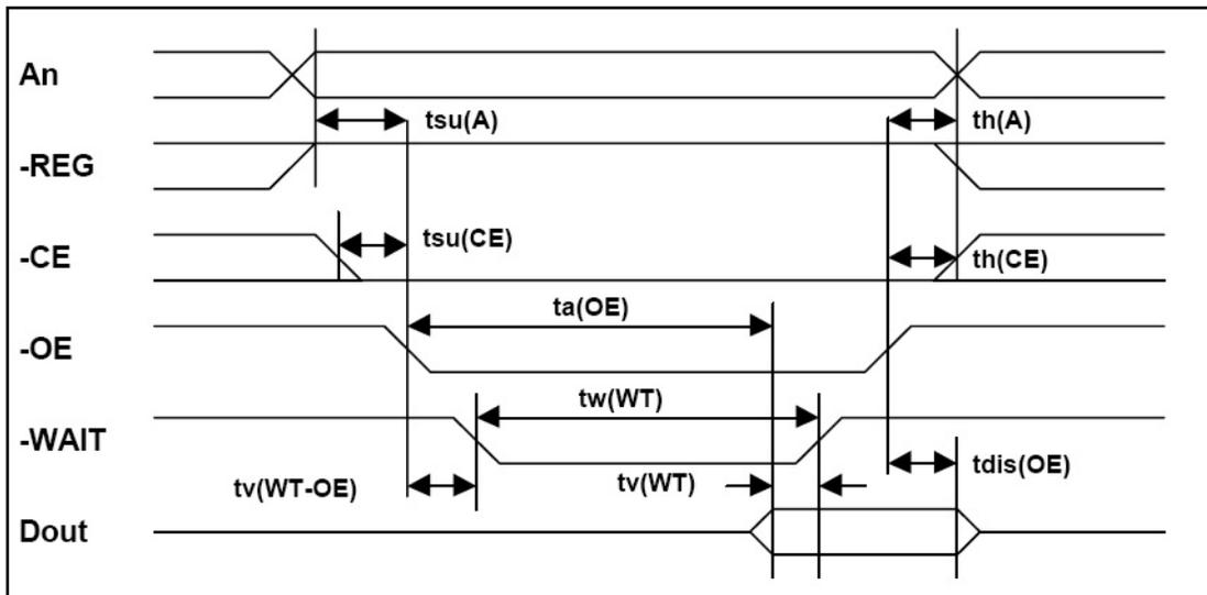
Figure 5: Timing Diagram of Common Memory Read
