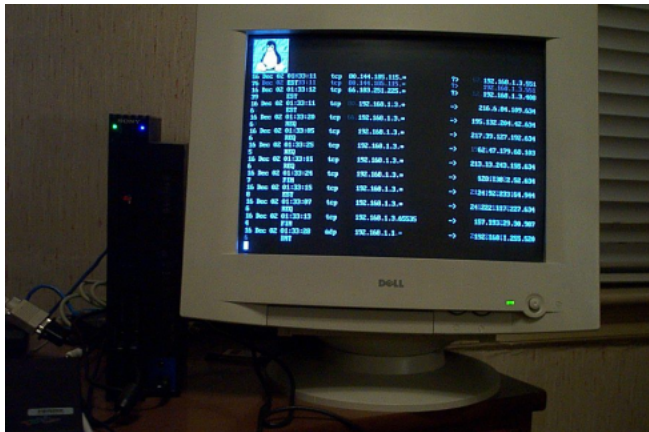
Figure 2: PS2 Network Analyzer in Action
