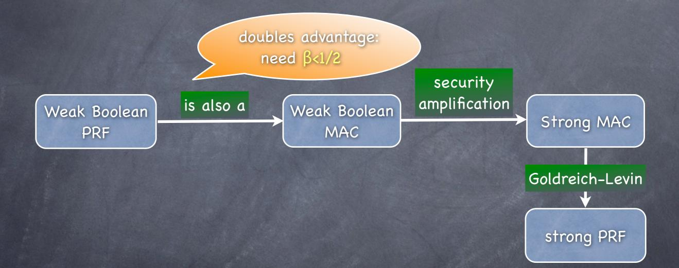
GL theorem does not work in general for showing MAC=>PRF [NR98] but works for our construction.
