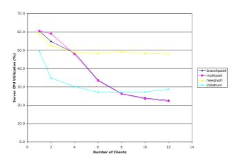
Figure 4: Web Test - Server CPU Utilization
