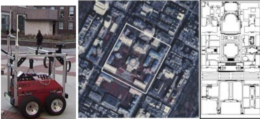
Fig. 1. The ATRV-2 Based AVENUE Mobile Robot (left), the outdoor campus environment as seen from above (center) and in outline form (right).
