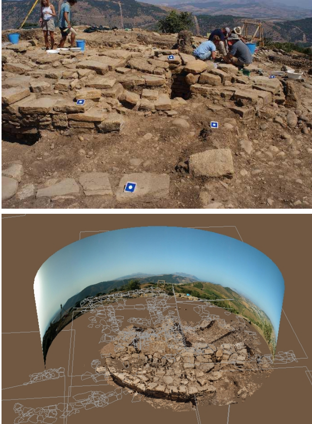
Figure 2. Modeling the acropolis at Monte Polizzo. Top: Targets have been placed in the area to be scanned. Bottom: Final textured model with panoramic image as background and GIS data.
