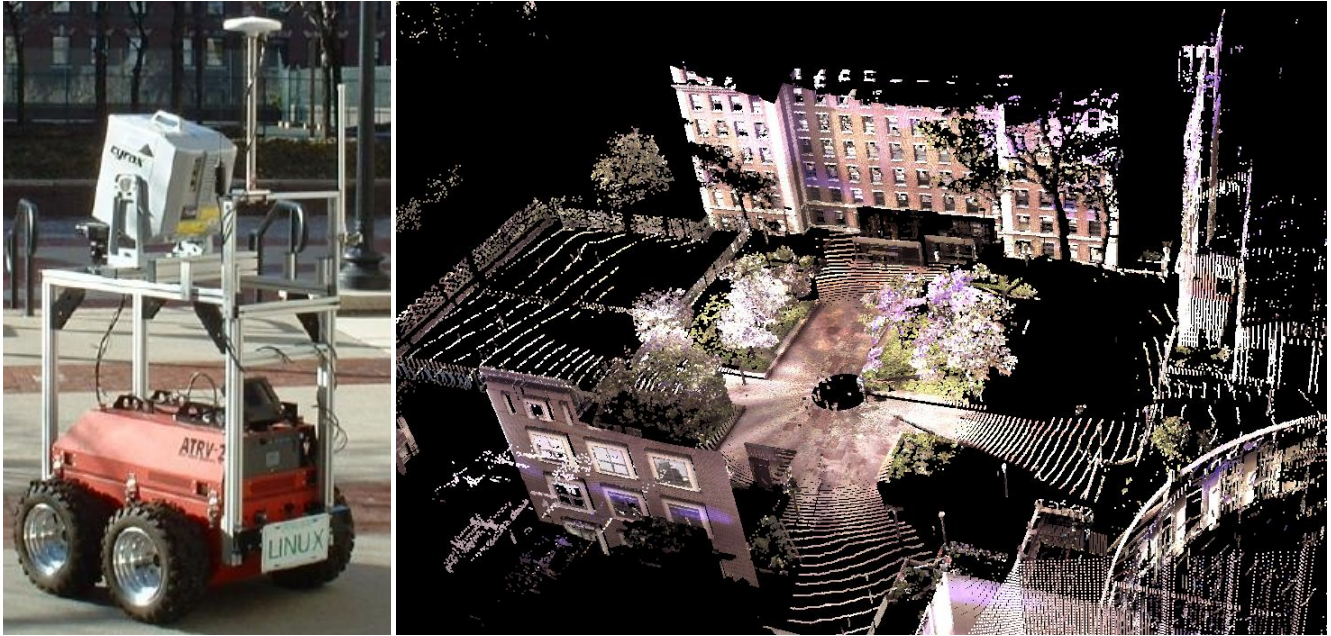
Figure 5. The ATRV-2 Based AVENUE Mobile Robot (left). A sample laser scan taken with the AVENUE system on the Columbia University campus (right). The hole at the center of the scan is where the scanner was positioned.
