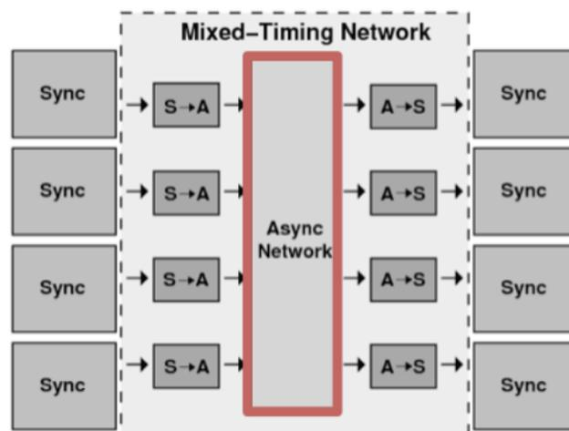
Asynchronous on-chip network integrating synchronous components
