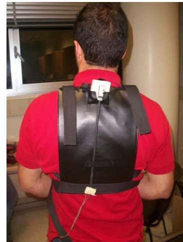
Figure 2. Spine stress monitoring system worn by patient
