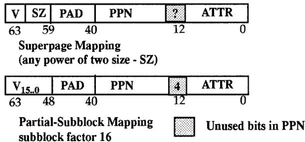
Figure 6: Superpage and Partial-subblock mapping format
