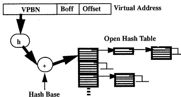
Figure 8: Storing partial-subblock and superpage PTEs in clustered page tables
