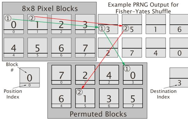
**Figure 3: Example of 8x8 block permutation.**
