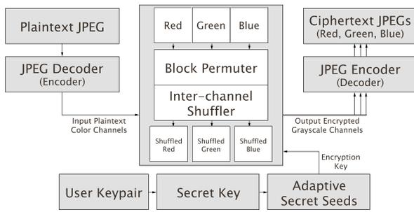
Figure 1: The ESP encryption architecture for JPEGs.
