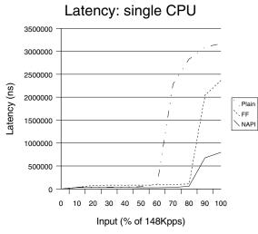
Figure 6. Latency results for single CPU
