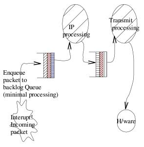
**Figure 1. Linux IP Forwarding path**
