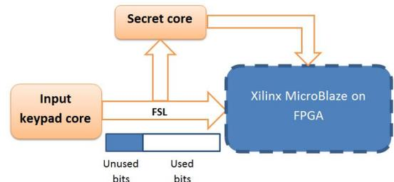
Fig. 3. Block diagram of a secret core for an untrusted e-voting machine.
