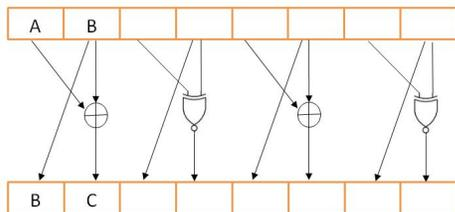
Fig. 5. Simple confusion function depending on data xoring.
