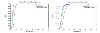
**Fig. 4.** Cumulative distribution function of all measured resolutions, for both the single-channel and the 4-channel version of the ARC, and for all different web applications. The majority of all request resolutions, about 98%, are completed in less than 10 microseconds.
