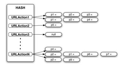
**Fig. 2.** The data structures used by ARC. A hash table, which holds references to linked lists hosting the set of the parameters of each schema. Each entry in the table has been produced by hashing the action part of a URL schema.
