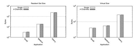
Fig. 6. Resident Set Size (RSS) and Virtual Size (VSIZE), both as reported by ps(1), while running ARC for each one of the three applications. Notice, that both, 4-channel and single-channel, versions have similar memory requirements. Also, memory requirements, in terms of RSS, from application to application increase linearly.
