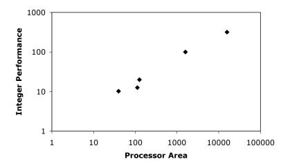
Figure 5: mpirical data confirming Pollack's rule, that processor performance
