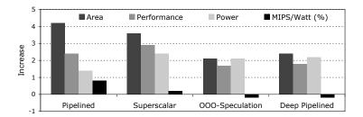
Figure 3: Area, performance, power, and efficiency effects of common ILPextraction techniques. Source: Shekhar Borkar, Intel.
