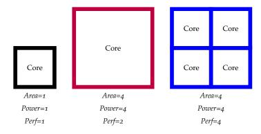
Figure 6: Spending Moore's law on multiple cores. Assume today's core (black) has unit power, area and performance. Quadrupling the transistor budget offers two options: scaling a single core (purple) or replicating the base core (blue). Because power scales with area, but performance with the square root of area, the multicore option (blue) offers a more power efficient option.
