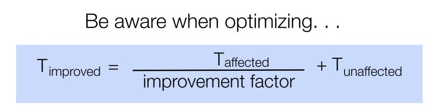
**Example:** On machine A, multiplication accounts for 80s out of 100s total CPU time.
