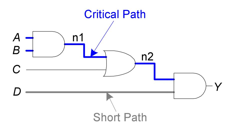
Critical (Long) Path:  $t_{pd} = 2t_{pd\_AND} + t_{pd\_OR}$ Short Path:  $t_{cd} = t_{cd\_AND}$
