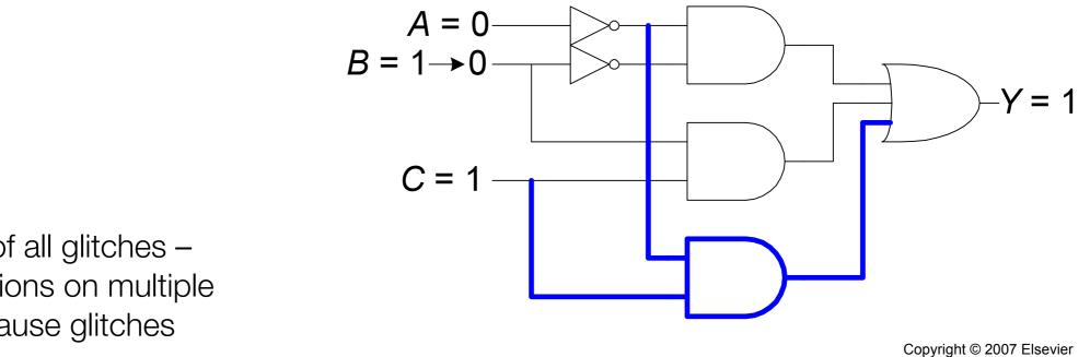
NB: Can't get rid of all glitches simultaneous transitions on multiple inputs can also cause glitches
