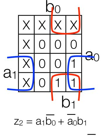
$(vs. a_1 \overline{a_0} b_1 + a_1 b_1 \overline{b_0})$
