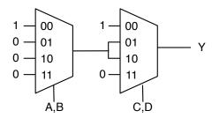
$$Y = \overline{C} \cdot \overline{D} + \overline{A} \cdot \overline{B} \cdot (C \oplus D)$$
