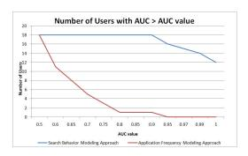
Fig. 4. The number of user models with AUC values greater than the value displayed on the x-axis for the search behavior and the application frequency modeling approaches using one-class SVMs. (The upper-left point shows 18 user models with AUC scores greater than 0.5)
