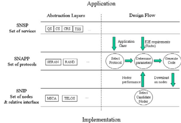
Fig. 2. Layers of abstraction and design flow
