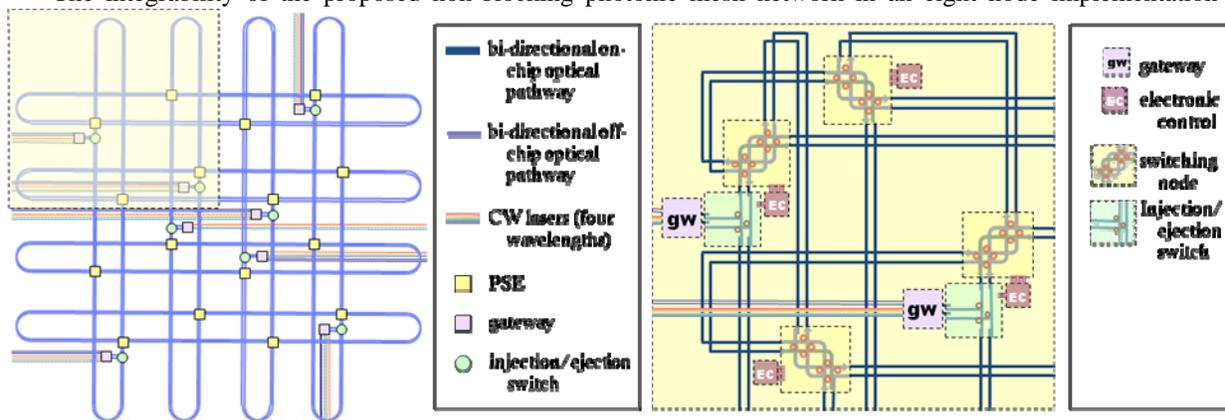
Fig. 2: Detailed layout of highlighted slice in the 8-port non-blocking photonic NoC
