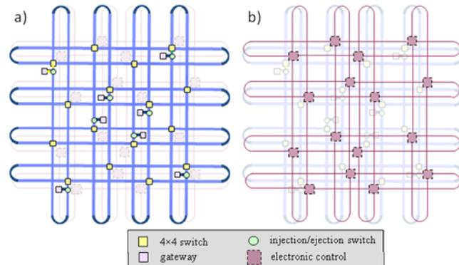
Fig. 2: (a) 8-port photonic NoC organization. (b) The associated electronic network
