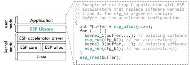
Figure 4: ESP accelerator API for seamless shared memory.
