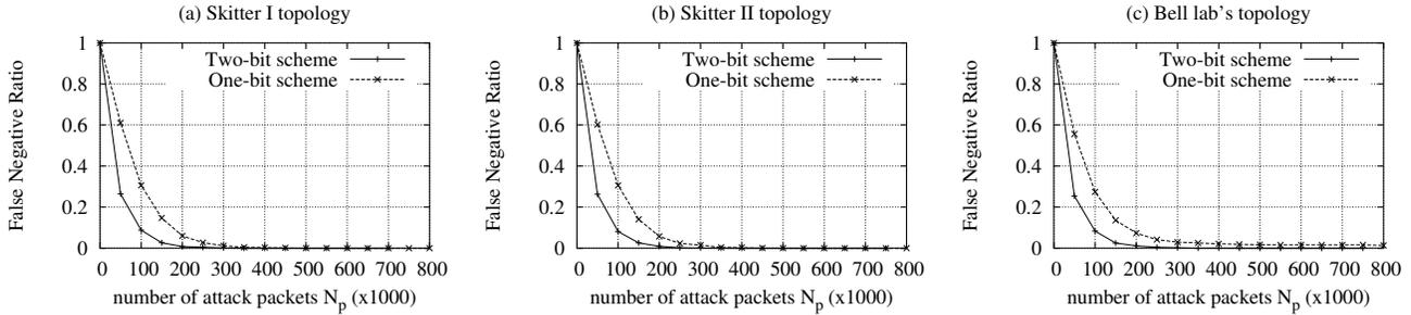
Fig. 10. False Negative Ratio of two traceback schemes on three different topologies
