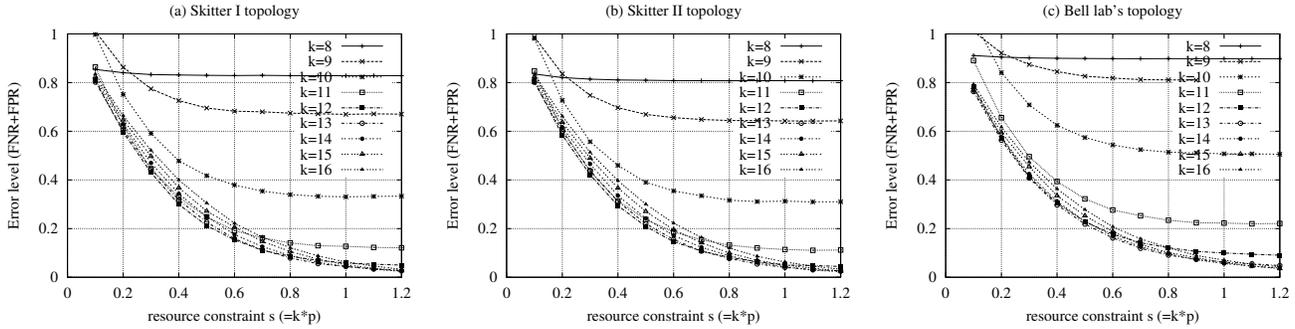
Fig. 5. Simulation results supporting the theoretical analysis (error level by varying  $s$ )
