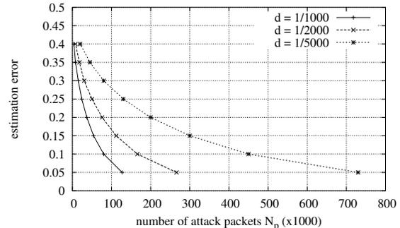
Fig. 3. The trade-off between the estimation error  $p_e$  and  $N_{min}$ , given  $s = 0.4$  and  $k = 12$ .
