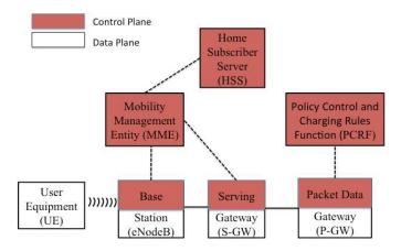
Fig. 2. Simplified LTE network architecture
