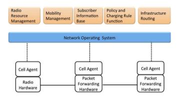
Fig. 3. Cellular SDN architecture
