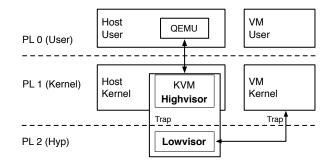
Figure 2: KVM/ARM System Architecture
