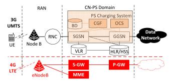
Figure 2: 3G/4G network architecture and charging components in PS domain.
