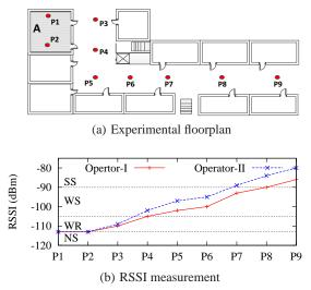
Figure 5: Our indoor testbed, where room A is a dead zone (NS-zone) for both operators.
