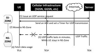
Figure 6: Procedure of DL-NS experiment.
