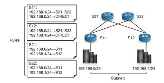
Figure 2: Small network example for describing the types of forwarding error found by Libra.
