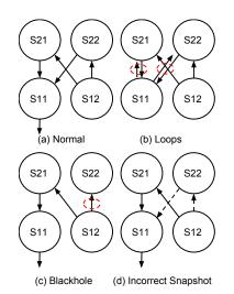
Figure 3: Forwarding graphs for 192.168.0/24 as in Figure 2, and potential abnormalities.
