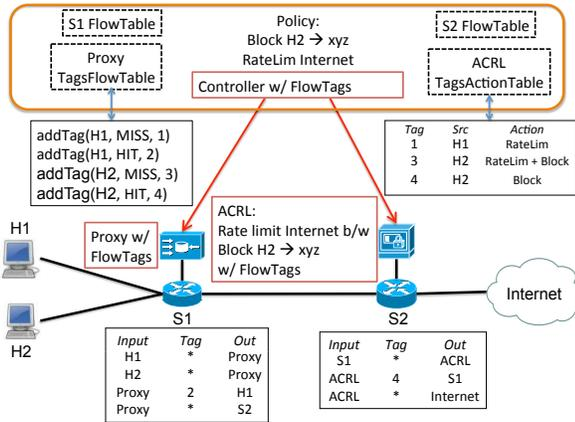
Figure 5: **An example of using FlowTags:** Each packet carries the contextual information necessary for correct policy enforcement (e.g., which source? is this cached or not?) Only the forwarding rules affected by tagging are shown for brevity.
