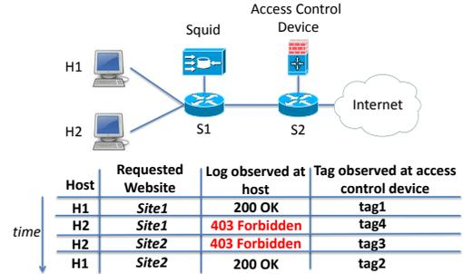
Figure 6: **Proof-of-concept:** The experiment shows that using Tags allows us to enforce the intended policy even in the presence of proxy effects. Tags also enable post-mortem verification to check if the policy was applied correctly.
