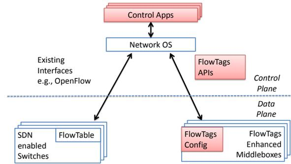
Figure 4: **The FlowTags architecture:** We highlight the extensions we introduce as part of FlowTags. We avoid explicit changes to switches or the need for direct interfaces between switches and middleboxes.
