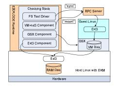
Figure 9: The VMware checking stack.
