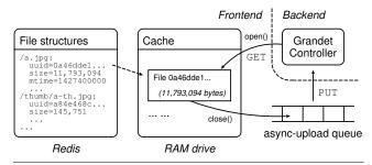
**Figure 7.** *Implementation of* GRANDET's file system interface. Solid arrows are the data flow. Dashed arrow shows the logical relationship between the file structure and its content.
