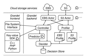
**Figure 4.** GRANDET *components*. Components with a plugin symbol mean that developers can easily extend them.
