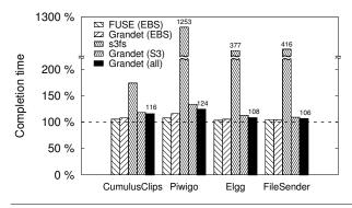
**Figure 12.** GRANDET's *end-to-end performance*. Time is normalized to the baseline which uses EBS directly.
