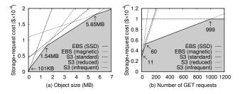
**Figure 1.** Monthly cost with (a) variable object size and (b) variable number of requests. Each line corresponds to a storage service. Assuming (a) has fixed 100 GET requests and (b) has fixed 1MB object size. Each request counts as one EBS I/O.
