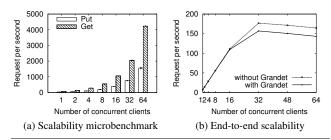
**Figure 13.** (a) *Scalability of* GRANDET *when using single S3 storages.* Evaluated with requests of 4KB in size. The error bar is the standard deviation. (b) *End-to-end scalability.* Evaluated on the FileSender application with real workload.
