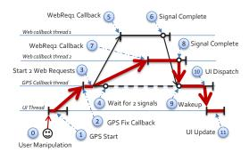
Figure 3: Execution trace of a location-based app.
