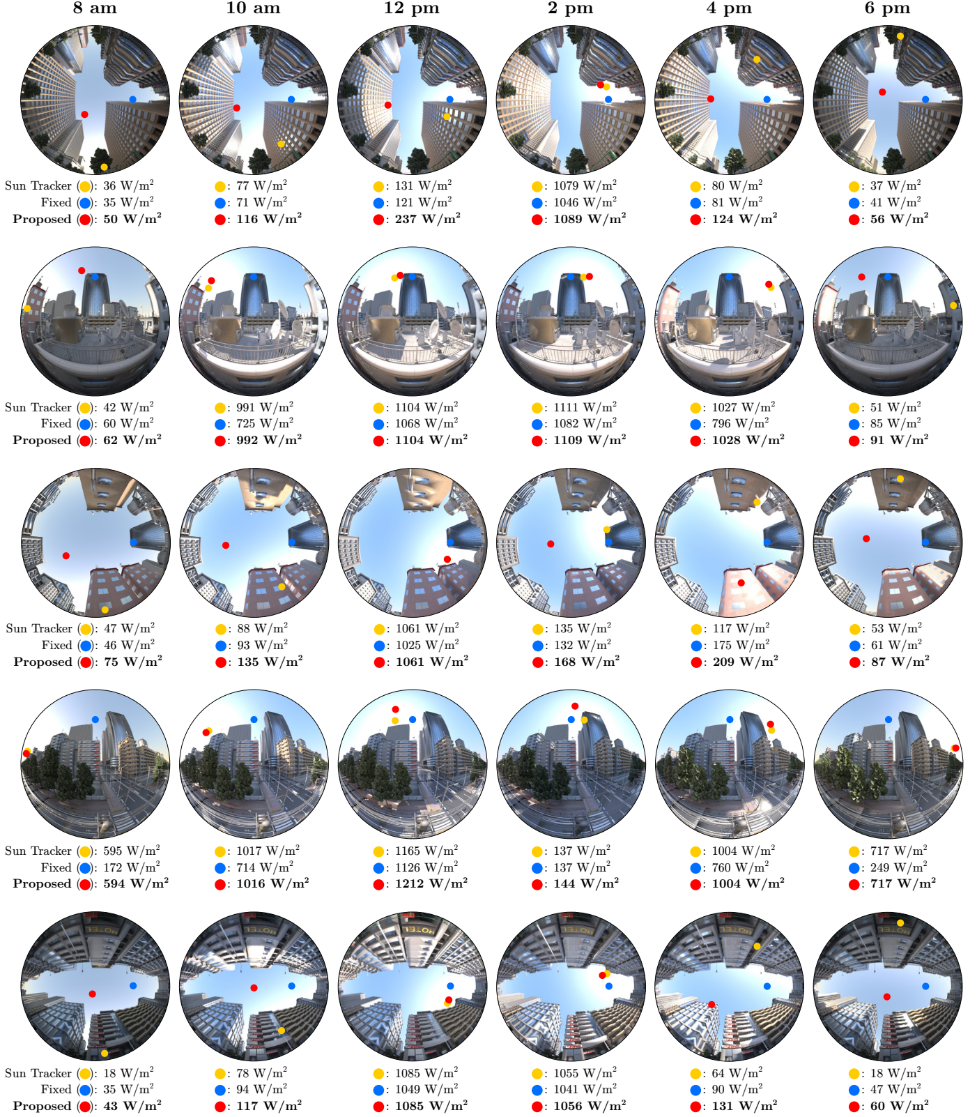
Figure 9: Simulations using dynamic illumination. We used a physically based renderer to simulate the illumination of a solar panel in dense urban settings over a single day. We randomly chose 6,137 different solar panel positions that represent typical urban solar panel installations. Each row shows the illumination at a single location at different times of day. Notice that as the sun moves through the sky, the illumination of nearby buildings and objects can change dramatically. Every 10 minutes, we simulated the energy harvested by a solar panel oriented using our approach (Proposed). We compare its harvested energy with that of a panel that tracks the sun (Sun Tracker) and another in a fixed orientation (Fixed). In each scene, the orientations of the sun tracker, the fixed panel, and the proposed method are denoted using the yellow, blue, and red dots, respectively. We also include the irradiance of each solar panel below. Notice that across the diverse environmental illuminations shown here, the irradiance of the panel oriented using our approach (Proposed) is consistently higher than the irradiance of the other two panels.
