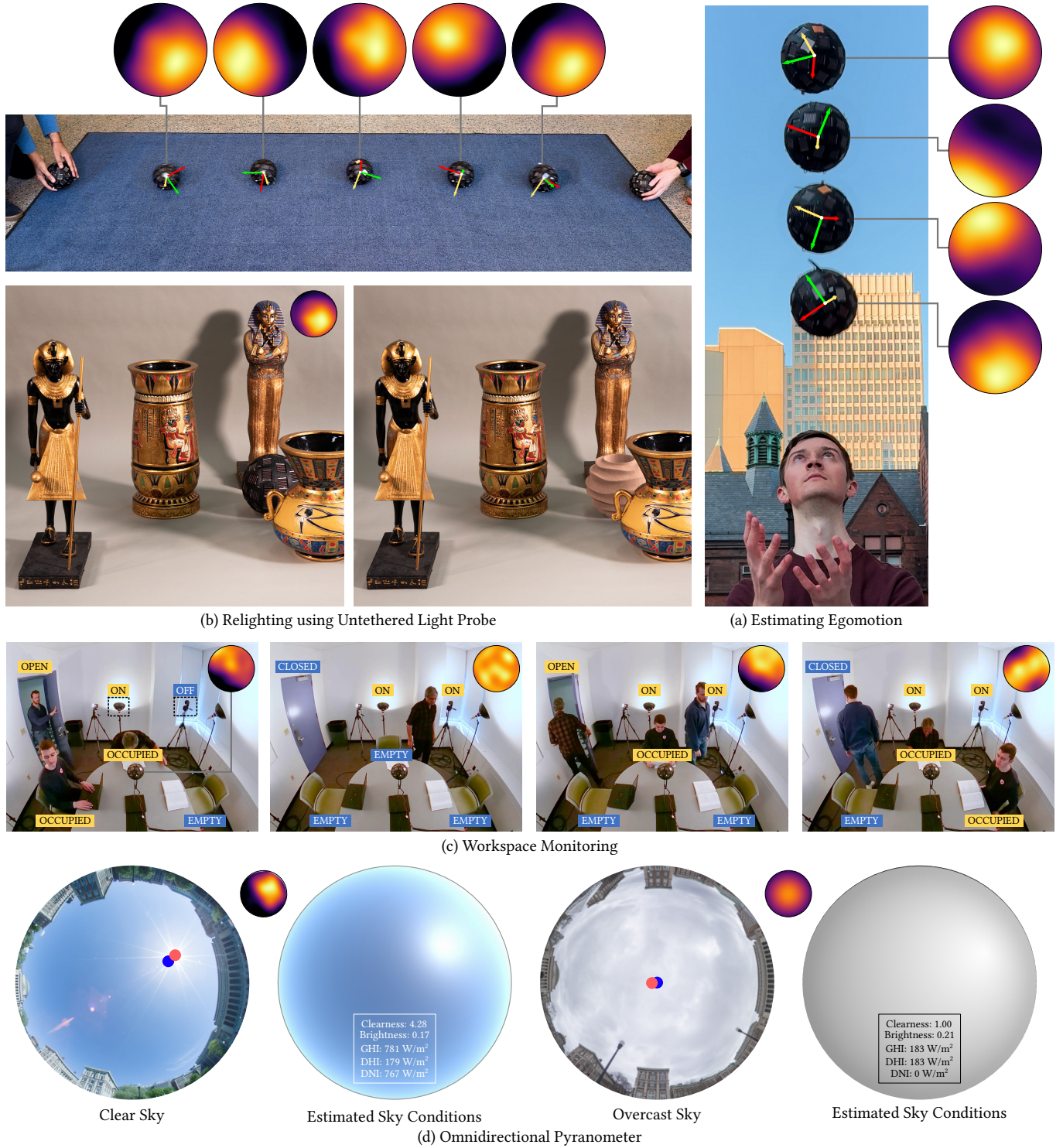
Fig. 11. Example applications of an irradiance camera. (a) FluxCam can be used as an optical gyroscope to determine the camera's orientation. Here we show the computed orientation as the camera is rolled across a floor and tossed in the air. (b) The camera can serve as an untethered light probe for diffuse relighting. We placed the camera in a location that is partially occluded by another object (left image) and measured the irradiance function (inset image). This allows us to relight and insert a diffuse object (right image). (c) FluxCam can be used to monitor a workspace. Here we use the camera's 49 measurements to determine which desks are occupied, detect when the door is open, and determine which lights are on (dashed black boxes in the left image). (d) FluxCam can be used as an omnidirectional pyranometer to estimate the best orientation of a solar panel (red dots). Additionally, the measurements can be used to reconstruct the sky, allowing us to quantify the current sky conditions. Please see the supplemental video.
