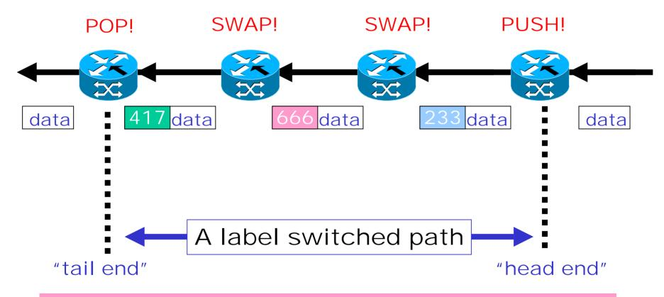
Often called an MPLS tunnel: payload headers are not Inspected inside of an LSP. Payload could be MPLS ...
