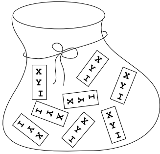
Figure 1. The bag of tuples representation for images. Each tuple encodes the (x, y) coordinates of a pixel and the corresponding intensity value.
