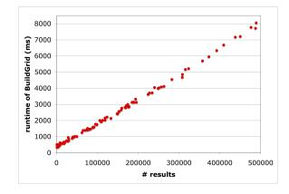
Figure 5.2: Execution time of **BuildGrid** as a function of dataset size.
