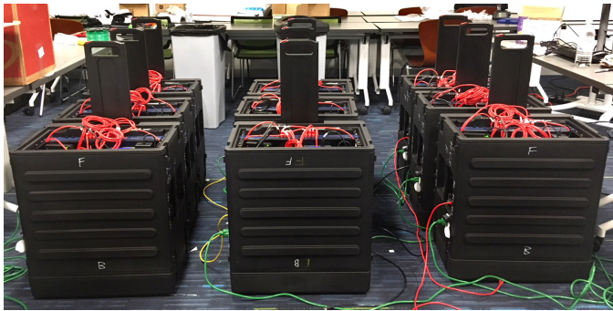
Fig. 12. Nine PhoenixSEN nodes set up in a lab at the University of Illinois at Urbana-Champaign. The full PhoenixSEN prototype consisted of 21 nodes.
