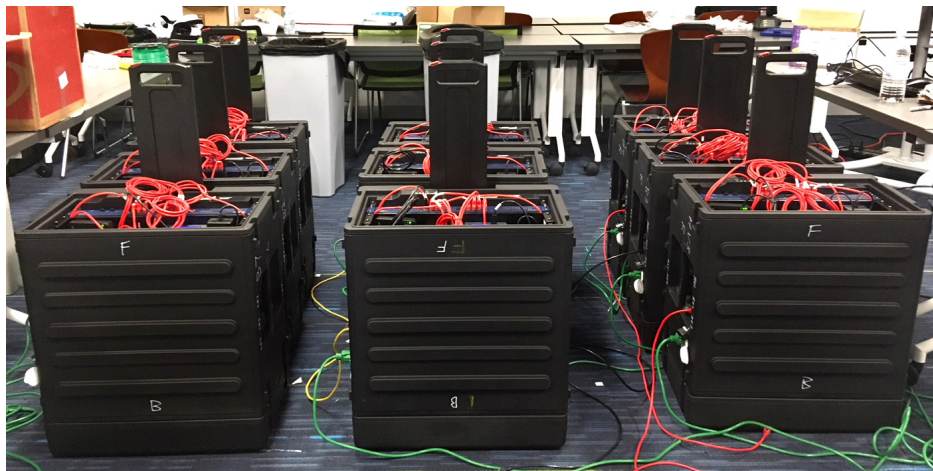
Figure 3.5: A portion of the PhoenixSEN prototype set up in a lab at the University of Illinois at Urbana-Champaign, September 2018. Each weather-resistant enclosure contains all the hardware for a single PhoenixSEN node. Photo author: Hema Retty. Used with permission.
