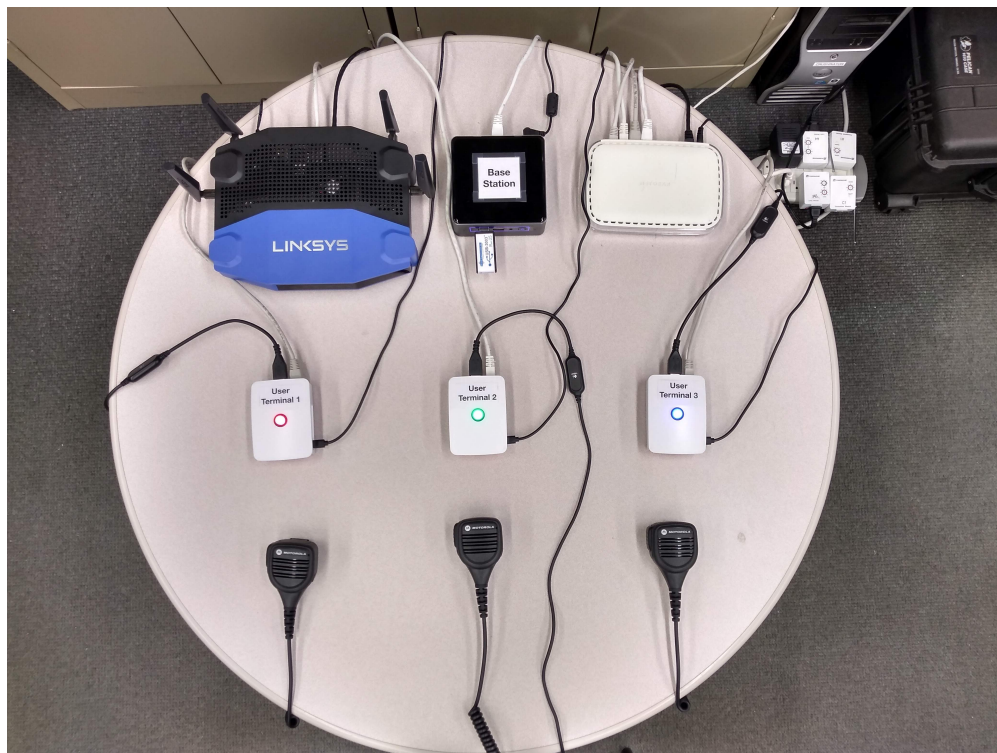
Figure 5.3: A photo of the mission-critical voice testbed built at Columbia University and used in all human-subject studies.
