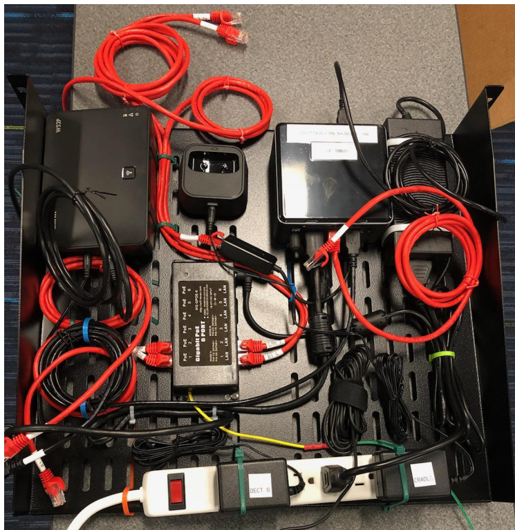
Figure 3.7: PhoenixSEN node components (Intel NUC, POE switch, Yealink W52P phone). September 2018. Photo author: Hema Retty. Used with permission.
