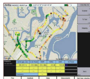
Over-the-Air On-screen Mapping Import map area on instrument screen to drive test downlink coverage of S-SS Power, RSRP, RSRQ, or SINR.
