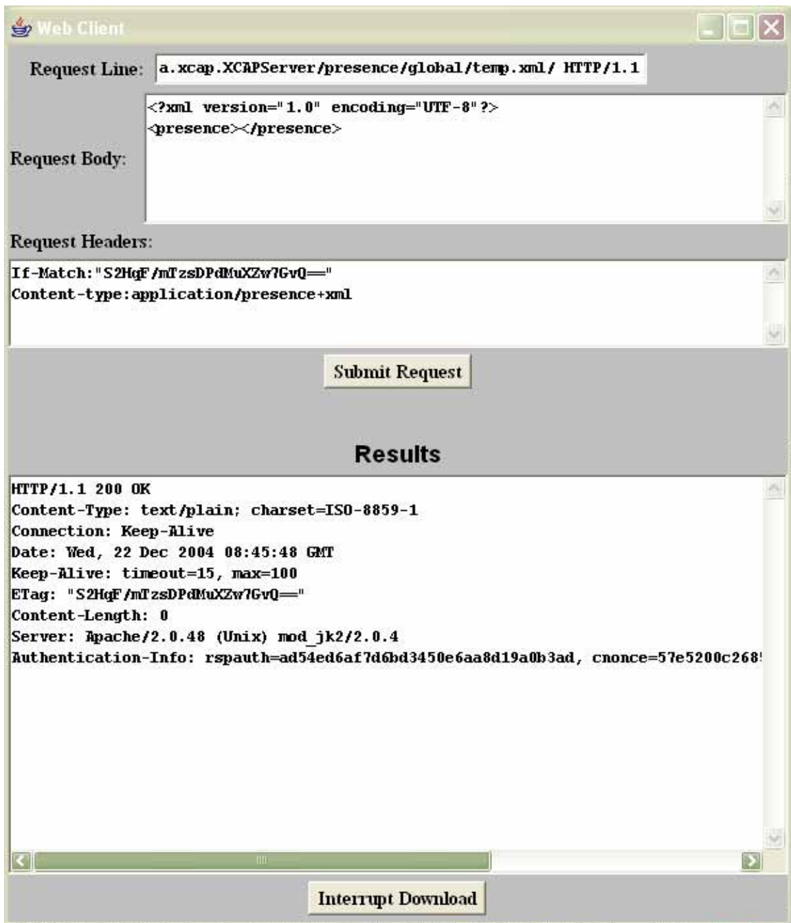
Figure 5: Same request tried after sending the If-Match header along with etag succeeds as Etag matches
