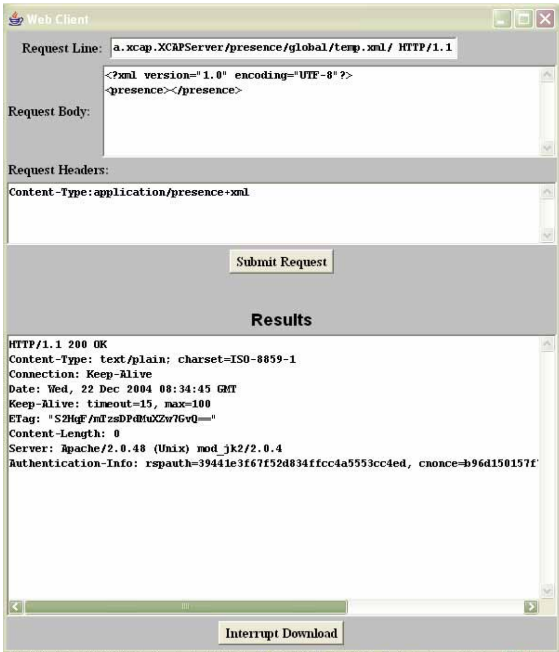
Figure 4: PUT request succeeded. Please note the content type as well as the ETag in the response that can
