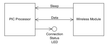
Beacons transmit a message at a predetermined interval of time that is broadcast to all tags within range. In addition, beacons indicate whether or not they can communicate with the network via the Connection Status LED.
