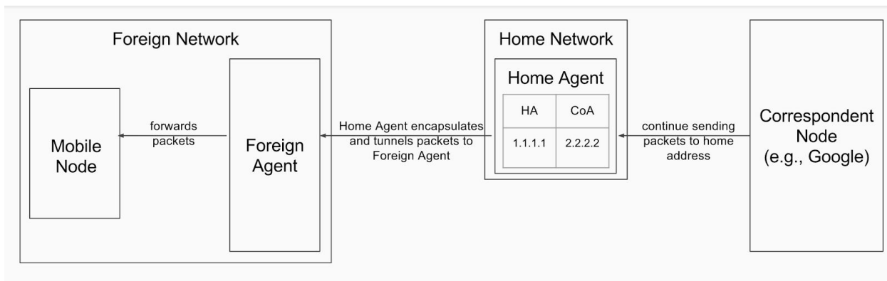
Figure 2. MIP in bidirectional tunneling mode
