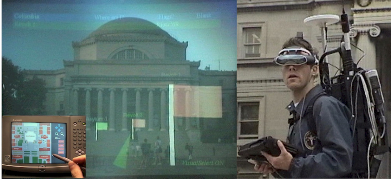
Figure 7: The Columbia Touring Machine. Mobile outdoor user wearing backpack and see-through head-worn display (right) sees strategic information overlaid on the real world (left). Complementary material is presented on a hand-held computer (lower left).
