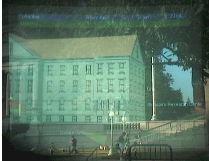
Figure 8: Model of demolished building, imaged through see-through head-worn display.
